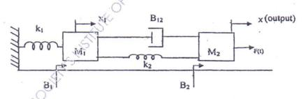
(b) Draw a signal flow graph for the system shown in fig 11a (ii) and hence obtain the transfer function using Mason's gain formula.
